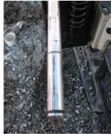
Figure 7: Seismic Cone Probe with 3 Triaxial Geophones and 1 Hydrophone
