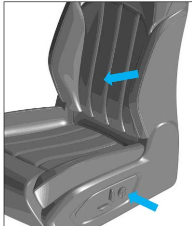
Toggle the round button on the side of the seat to adjust the lumbar area of the backrest up and down and back and forth to enhance lumbar comfort.
