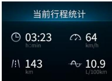
Record the current trip fuel consumption, speed, mileage and time, long press the steering wheel OK button to reset and clear some information.
