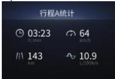
Record the fuel consumption, speed, mileage and time of trip A. Press and hold the steering wheel OK button to reset and clear some information.
