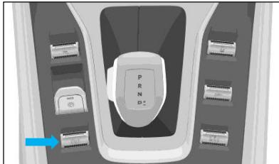
▷ Press the Auto hold switch to turn on the automatic parking function. At this time, the auto hold function is in the ready state and the indicator light <sup>Auto</sup> <sup>hold</sup> on the combination meter is on.
