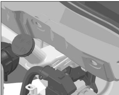
Visually check the fluid level without removing the lid by looking at the external markings on the side of the reservoir. The brake fluid level should be between
