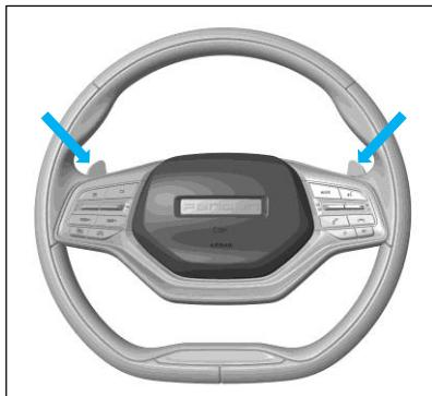
When the automatic gearshift is electronic, the shift paddles are used for manual mode driving, and the shift paddles on the steering wheel are plucked to manually upshift or downshift.
