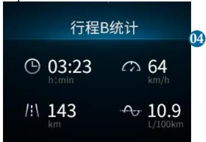
Record the fuel consumption, speed, mileage and time of trip B. Press and hold the steering wheel OK button to reset and
