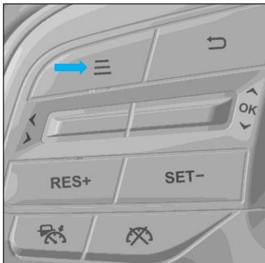
Press the button
