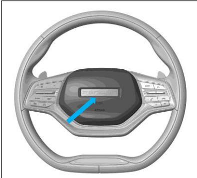
To sound the horn, press the center flap on the steering wheel.
