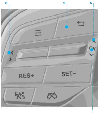
In any interface, you can switch the first-level menu by dialing the screen selection key on the left side of the multifunction steering wheel up and down. If you do not operate for 2s, the current content will be selected by default, the menu bar will be hidden, and the menu will not be cycled.
