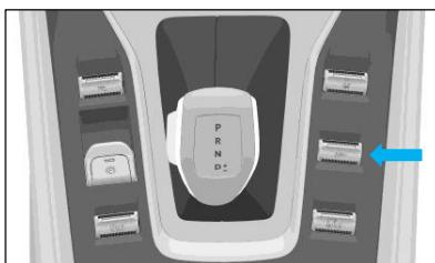
The hill descent system is an auxiliary system that can help the driver to go down the hill slowly, for example, when driving and reversing on a steep slope or on a mountain road in winter.
