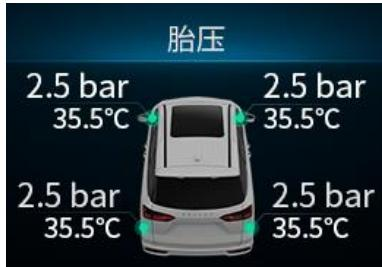
Tire pressure and temperature can be fed back to the gauge via the tire pressure sensor and displayed in real time on the gauge display.
