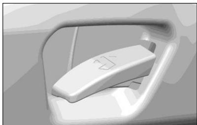
Pull the backrest release handle upward to adjust the angle of the backrest; directly pull the backrest release handle up completely to flatten the backrest, then release the handle. ( Manual adjustment )
