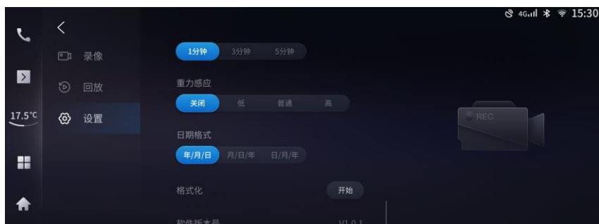
The touch screen can set the parameters of the driving recorder. In the real-time preview interface, touch the setting button on the left to enter the setting interface, where you can customize settings for resolution, loop recording, gravity sensing, date format, formatting, etc.
