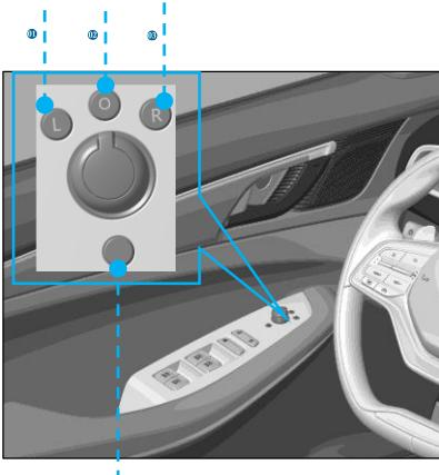
1. Adjustment of exterior rearview mirror: rotate the switch to select or (left or right), and toggle the adjustment knob to adjust the angle of exterior rearview mirror lens;;
