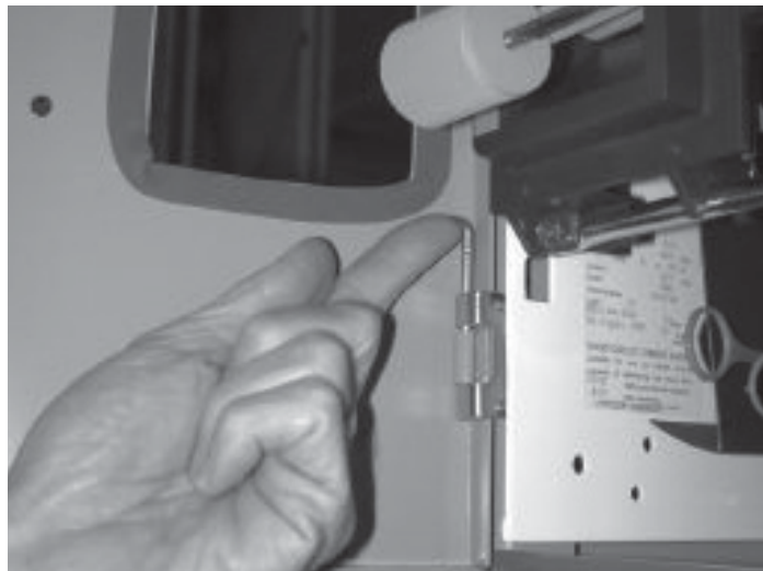
Figure 29. Hinge pin removal
