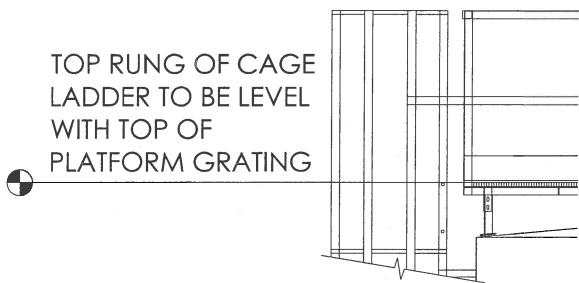
SAFETY CAGE/PLATFORM ELEVATION
