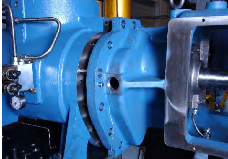
Figure 5-17: Separating Gear Housing from Compressor
