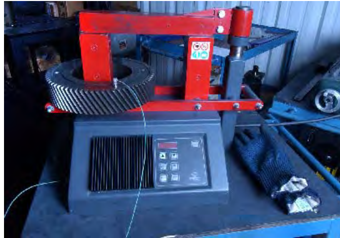
Figure 5-22: Heating New Gear
