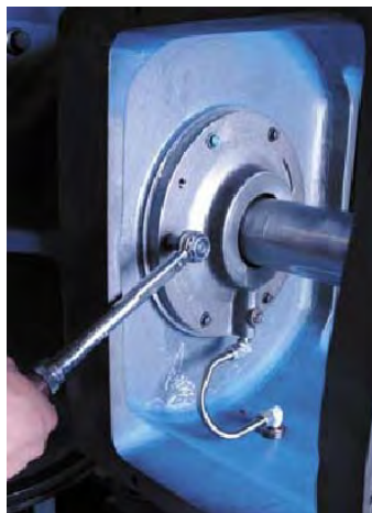
FIGURE 5-7: INSTALLING SEAL HOUSING & TUBING
