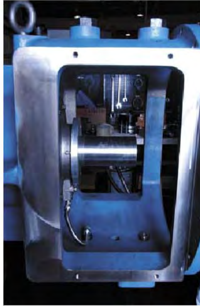
FIGURE 5-2: INSTALLING SEAL HOUSING REMOVAL/INSTALLATION TOOL
