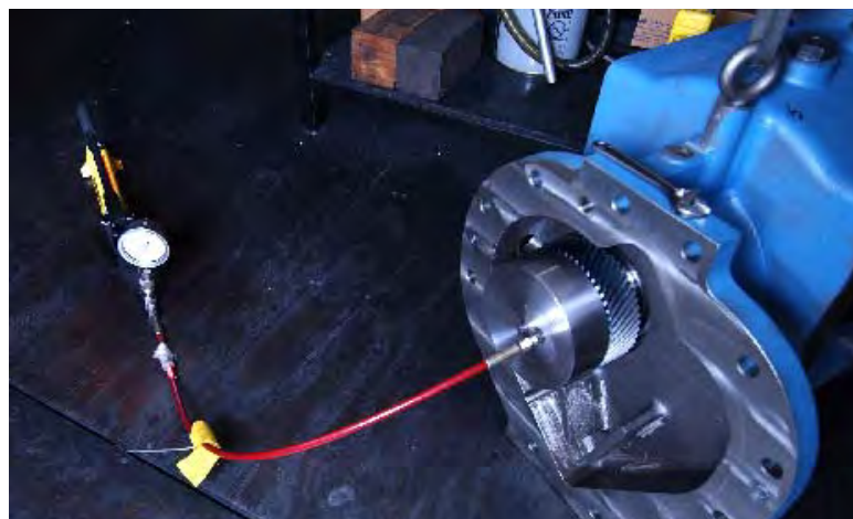
Figure 5-20: Pressurizing to Remove Gear
