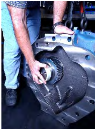
Figure 5-18: Installing Plastic Protective Sleeve Tool
