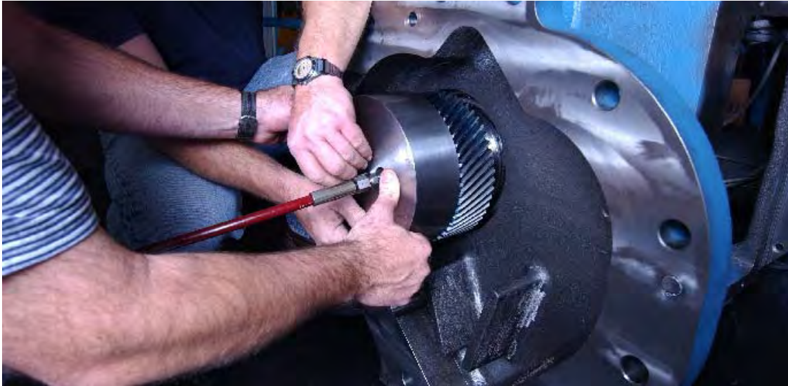
Figure 5-19: Installing Gear Stop/Retainer
