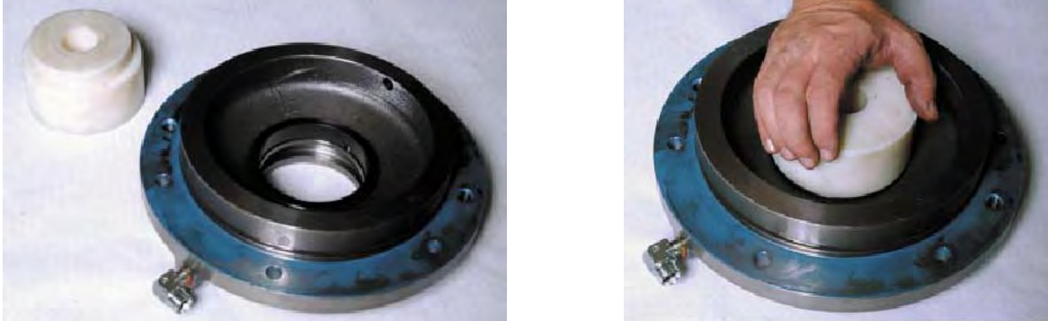
FIGURE 5-6: INSTALLING STATIONARY HALF OF SEAL
