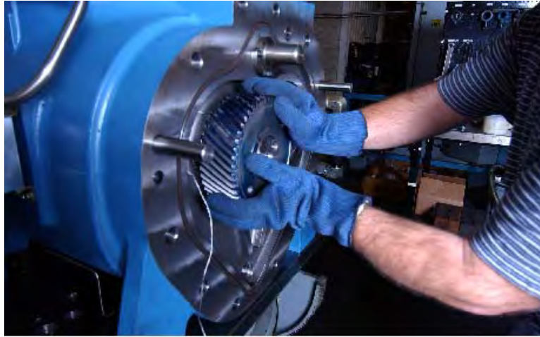
Figure 5-24: Installing New Pinion
