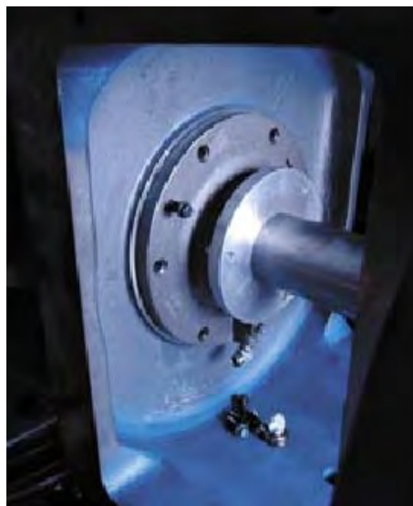
FIGURE 5-3: LOOSENING & REMOVING SEAL HOUSING & TOOL
