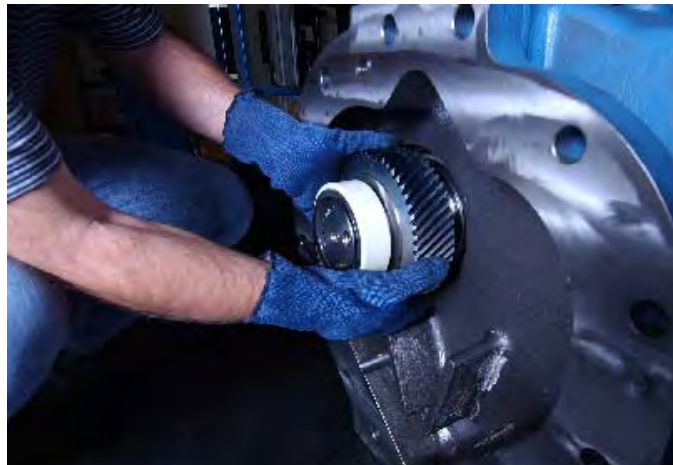
Figure 5-23: Installing New Gear
