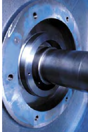
FIGURE 5-4: ROTATING HALF OF SEAL REMOVED
