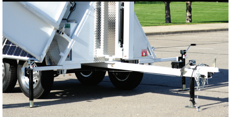
Figure 11: Hybrid 1200 with Outriggers Deployed
