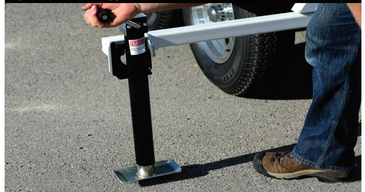
Figure 10: : Outrigger Arm Extended & Jack Stand Deployed
