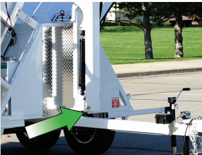
Figure 18: Mast Extension Lock located at the base of the mast while upright.
