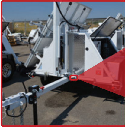
Figure 4: Tire Placard is located at the front of the unit at the bottom of the mast.
