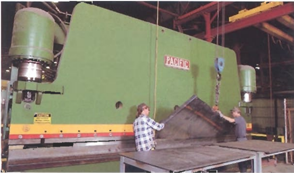
400 ton, 3/4" X 22' press brake
