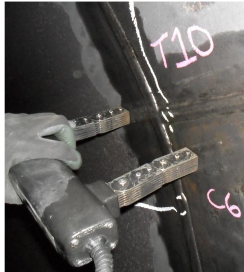
T10 / C6 - 2 Indications in the Start / Stop of the Weld
