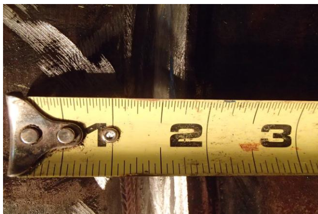
Grinding Width Approx. 19.05 mm Wide x 4.45 mm Deep
