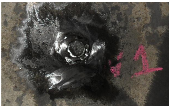
N1 - 2 Indications Just Below the Nozzle Weld
