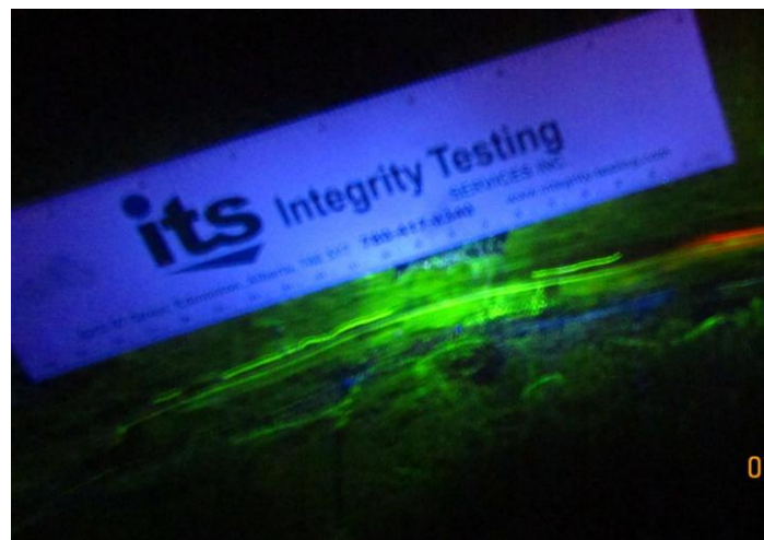
West Head Crack In - Between WHT3 and WHT4
