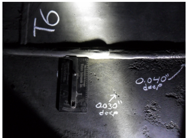
Photo 6: Corrosion on East End
