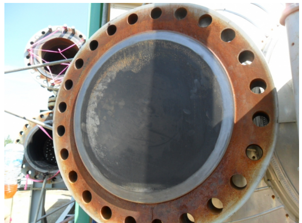
Photo 12: Manway Cover Plate and Sealing Area
