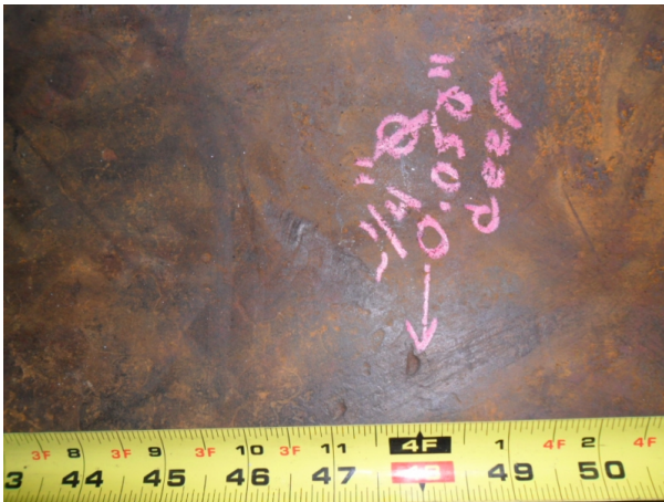
Photo 19: Pitting and Mechanical Gauges (3)
