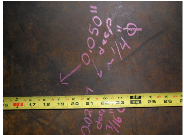
Photo 20: Pitting and Mechanical Gauges (4)
