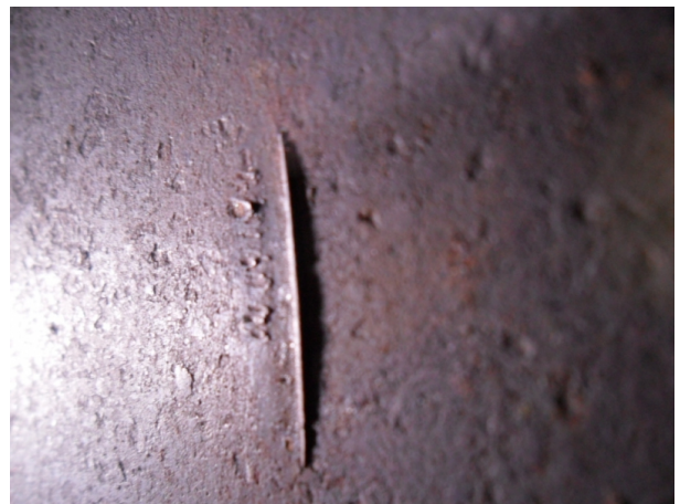
Photo 18: Pitting and Mechanical Gauges (2)
