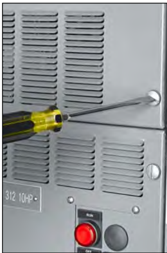
Figure 90 – Loosening Captive Fasteners
