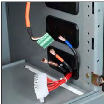
Figure 94 – Power Leads and Top of Terminal Blocks Fed Through Wiring Port
