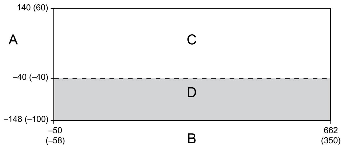
**Ambient and process temperature limits for Super Duplex ELITE meters**
