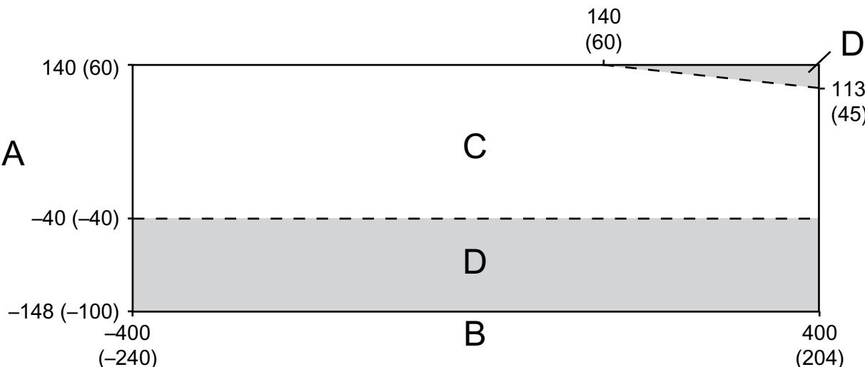
**Ambient and process temperature limits for ELITE CMFS025–CMFS150 meters**
