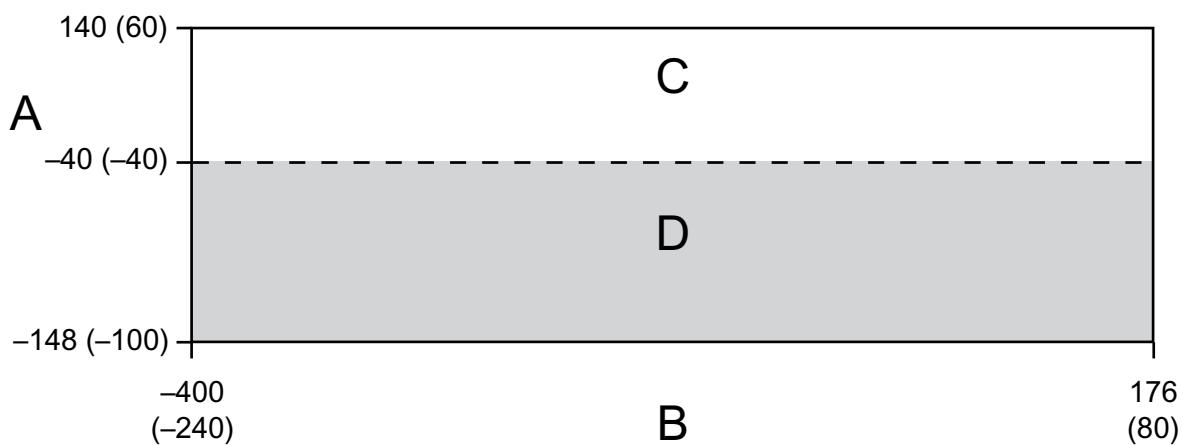
**Ambient and process temperature limits for high temperature ELITE meters**
