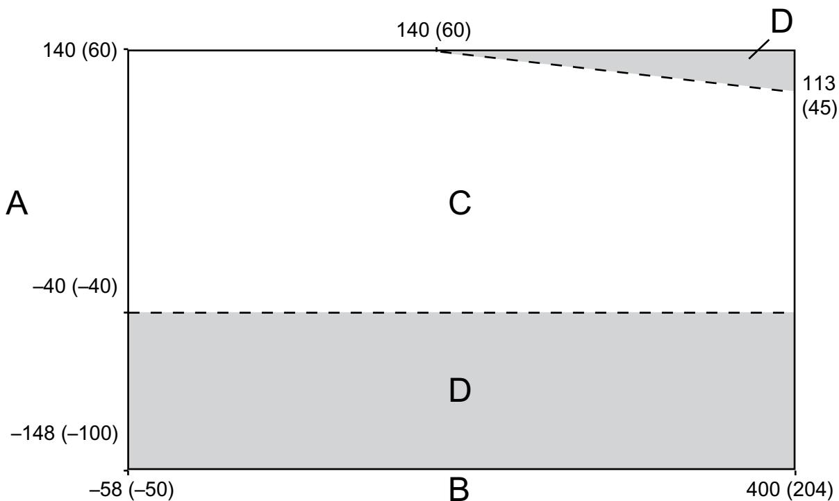
**Ambient and process temperature limits for cryogenic ELITE meters**
