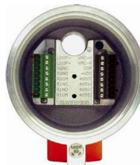
Figure 11 – CLASSIC 800 Mounting Base Plate / Wiring Terminal
