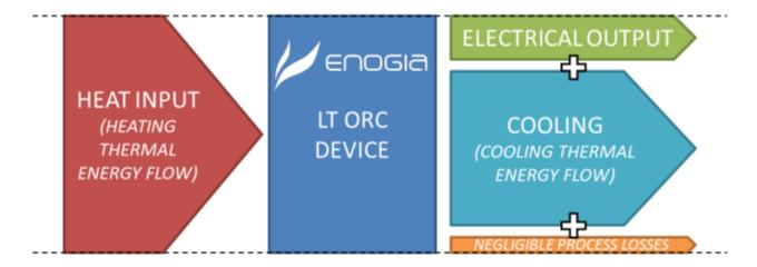
However, all the heat cannot be converted into electricity. The system has a system efficiency, which can be calculated by using the electrical output power, divided by the thermal inlet power.
