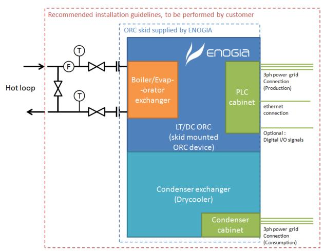
NOTA: the flow meters (F), the temperature sensors (T) and the bypass lines are recommended in order to monitor ORC performance and to ensure customer process running in case ORC is stopped, however they are not mandatory for ORC operation. The Digital I/O signals can be connected as an option.
