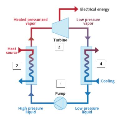
As the commonly used steam Rankine cycle, the Organic Rankine Cycle uses the discharge of high pressure fluid through a turbine expander in order to produce mechanical and electrical output (3).
