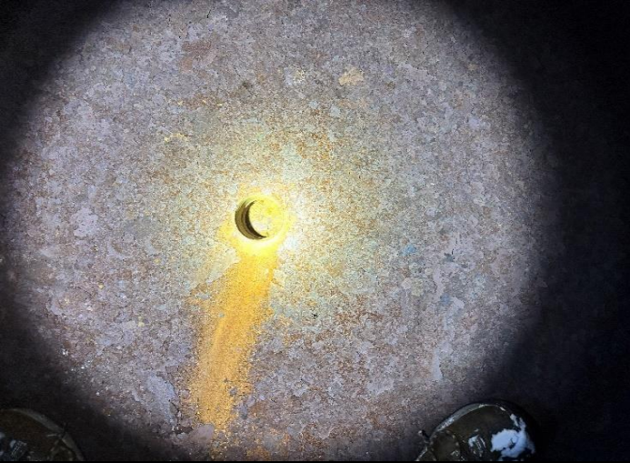
Photo 1: Surface debris in vessel welding good condition
