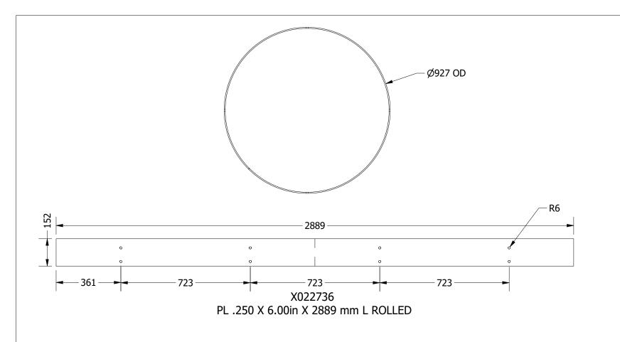
THESE HOLES ARE TO BE CUT AT THE TIME OF DRY FITTING - PRIOR TO GALVANIZING.
