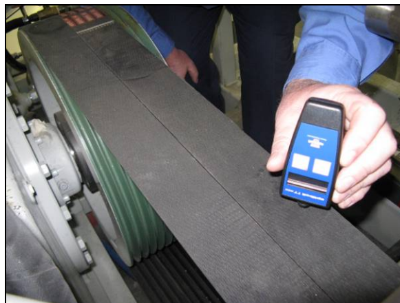
Figure 18: Example Orientation of Frequency-based Belt Tension Tester
