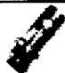
8201-001, Conduit Union Fits between transmitter and 8200-001 conduit elbow to facilitate installation and wiring where there is not enough room to rotate the elbow. Suitable for Class I, Div. 1 (Grps A, B, C & D) and Class II, Div. 1 (Grps E, F & G), hazardous areas. Material: zinc plated steel.
