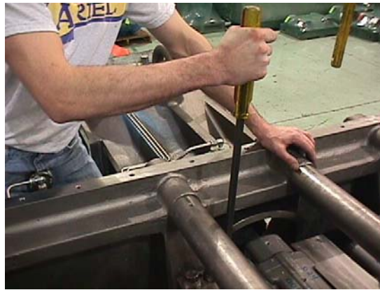
Use Large Screwdriver or Pry Bar against Compressor Frame, Thrusting Crankshaft Back & Forth
