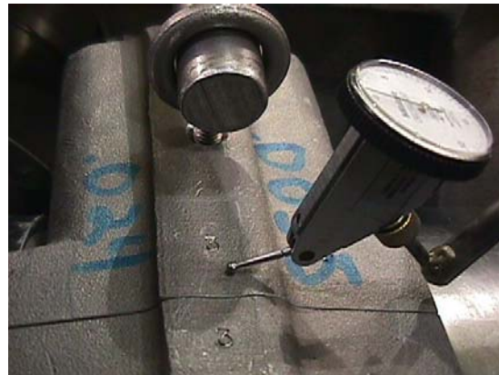
Needle Type Dial Indicator Placement on Top of Connecting Rod
