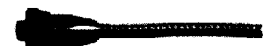
9334-211-YYYY-XXXX, Cable Assembly, w/Stainless Steel Armor Two (2) pin socket connector with 7.1 mm (0.28") diameter, SST armored jacket with cable, twisted shielded pair wires. xxx.x = Cable length in meters. yyy.y = Armor length in meters.
