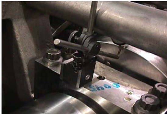
Dial Indicator Magnetic Stand Placement on Top of the Main Bearing Cap
