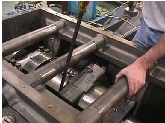
Rod Thrust Tight Away from Dial Indicator
