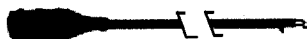
8978-111-XXXX, Splashproof Cable Assembly Two (2) pin socket connector with integral, molded splash proof boot with 6.4 mm (0.25") diameter polyurethane jacketed cable with twisted shielded pair wires. xxx.x = Cable length in meters.
