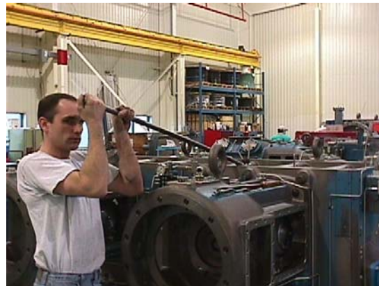
Using Pry Bar to Check Jack Clearance
