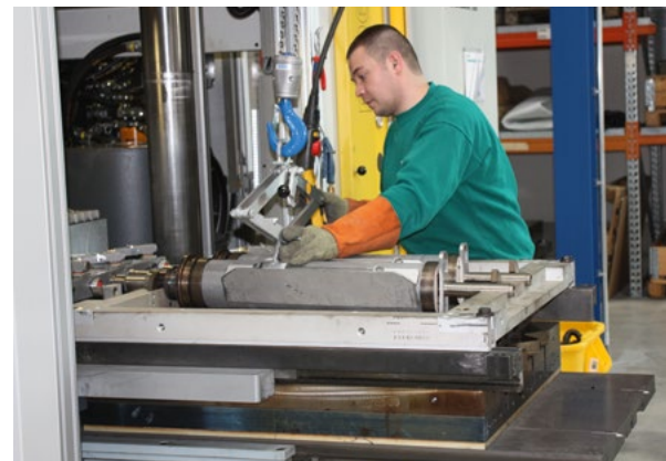
Injection moulding machine for iFD-stators®
