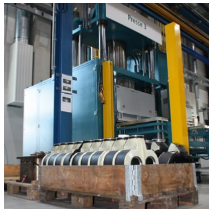
Press with casing liners for TORNADO® T2
