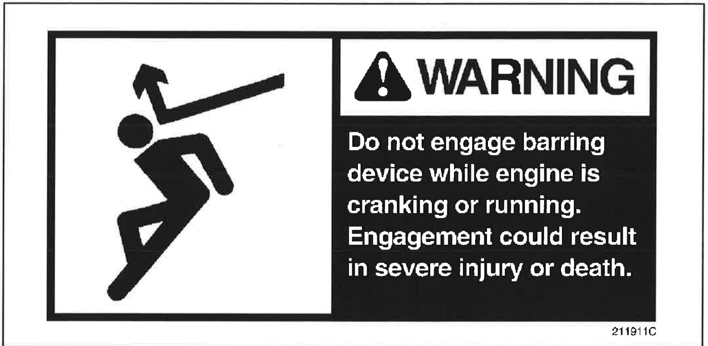
Figure 1.00-16. Warning Label - P/N 211911C - Barring Device
