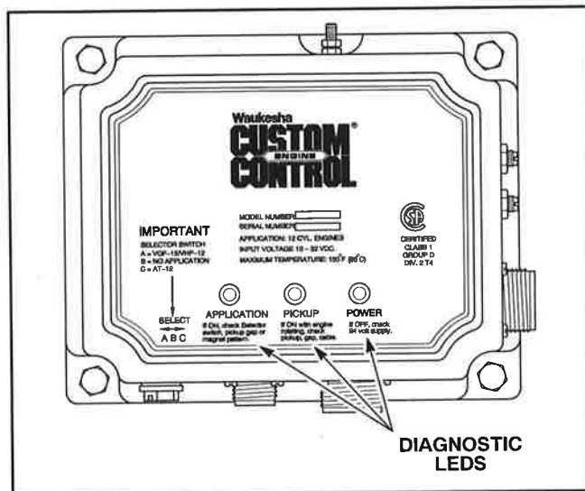
Figure 5.00-1. Ignition Module Diagnostic LEDs
