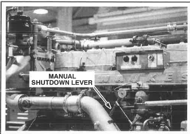
Figure 3.00-24. Manual Shutdown Lever - 6 Cylinder GSI Engine
