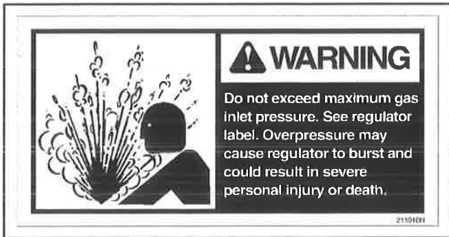
Figure 1.00-11. Warning Label - P/N 211910N - Maximum Gas Regulator Pressure
