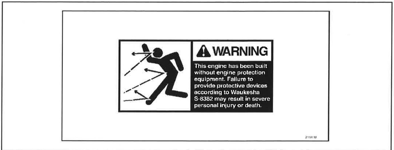
Figure 1.00-15. Warning Label - P/N 211911B - Built Without Engine Protection
