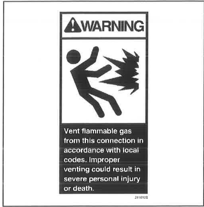
Figure 1.00-12. Warning Label - P/N 211910S - Vent Flammable Gas
