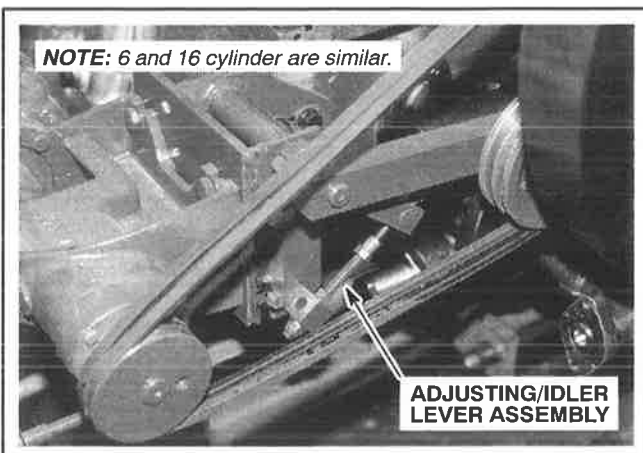
Figure 4.25-8. Adjusting/Idler Lever Assembly - 6 Cylinder Shown
