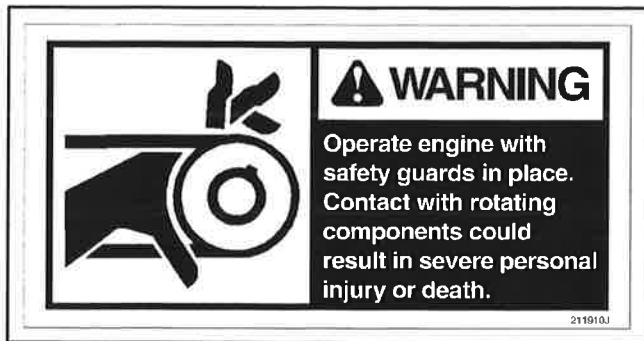
Figure 1.00-7. Warning Label - P/N 211910J - Safety Guard
