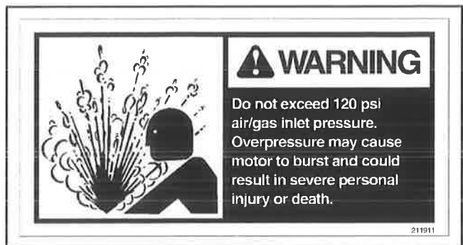
Figure 1.00-13. Warning Label - P/N 211911 - Maximum Air Prelude Motor Pressure
