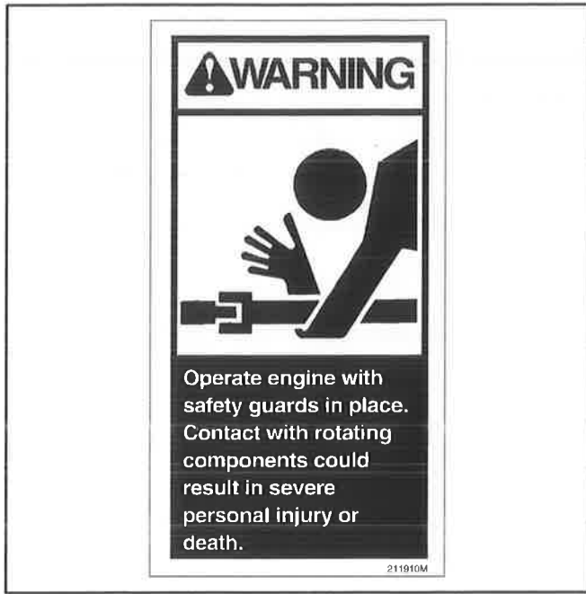
Figure 1.00-10. Warning Label - P/N 211910M - Safety Guard
