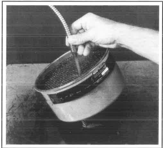
Figure 4.40-11. Wash Separator With Solvent
