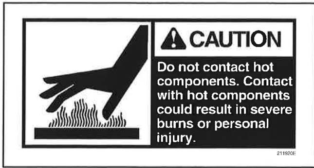
Figure 1.00-20. Caution Label - P/N 211920E - Hot Components
