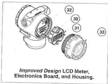
LCD Meter and Housing Exploded Views, Improved and Previous Design.
