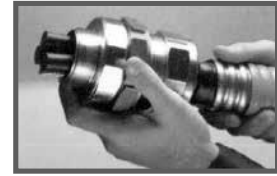
2. Install Star Teck XP® on cable
