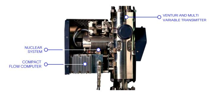
The Vx Spectra flowmeter is comprised of three sections: a venturi section and multivariable transmitter for measuring total flow rate; a nuclear source and detector that obtains oil, gas, and water holdups; and a compact flow computer that performs all calculations and converts flow measurements from line to standard conditions.
