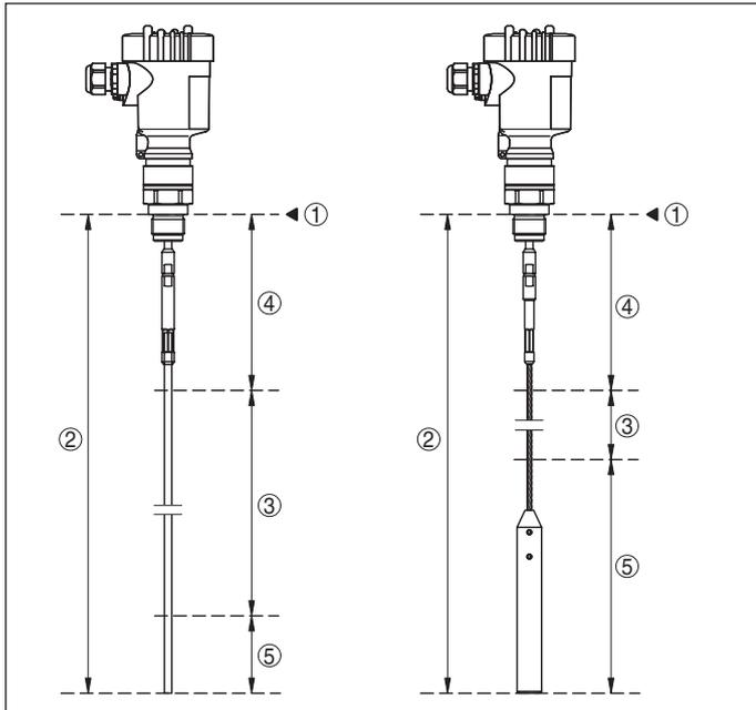
Fig. 1: Measuring ranges of the VEGAFLEX cable and rod versions
