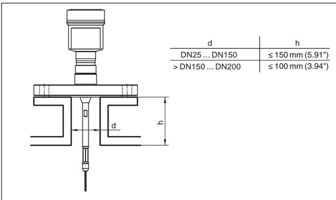
Fig. 16: Mounting socket
