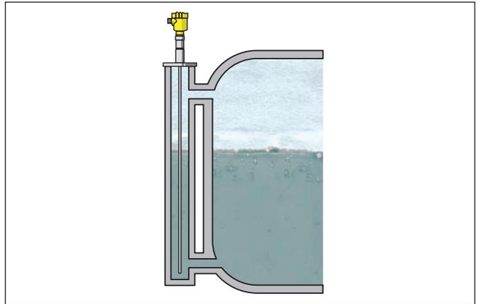
Fig. 30: Level measurement in a bypass tube
