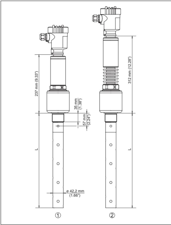
Fig. 59: VEGAFLEX 86, coax version with threaded fitting
