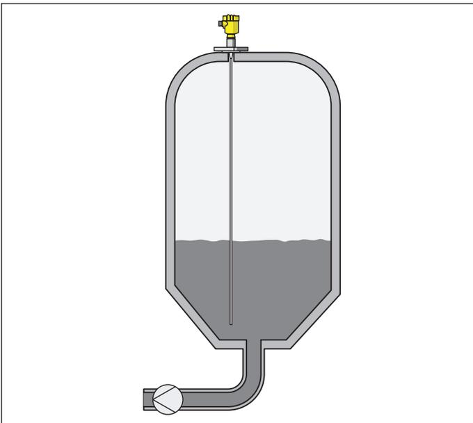
Fig. 29: Level measurement in a vessel with foodstuffs with VEGAFLEX 83
