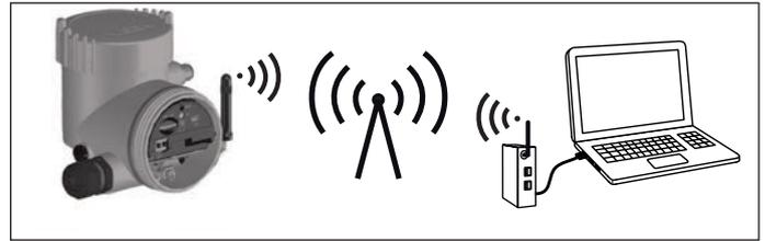
Fig. 50: Transmission of measured values and remote parameter adjustment of the sensor via mobile phone network.
