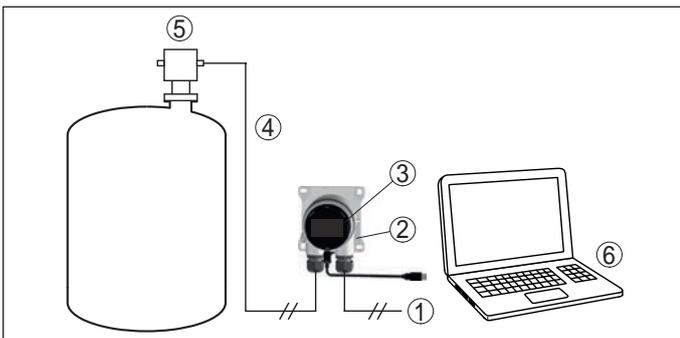
Fig. 49: Connection of VEGADIS 82 to the sensor, adjustment via PC with PACTware
