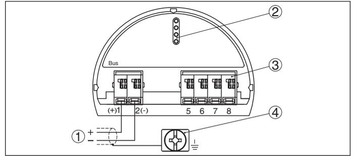
Fig. 36: Terminal compartment, double chamber housing
