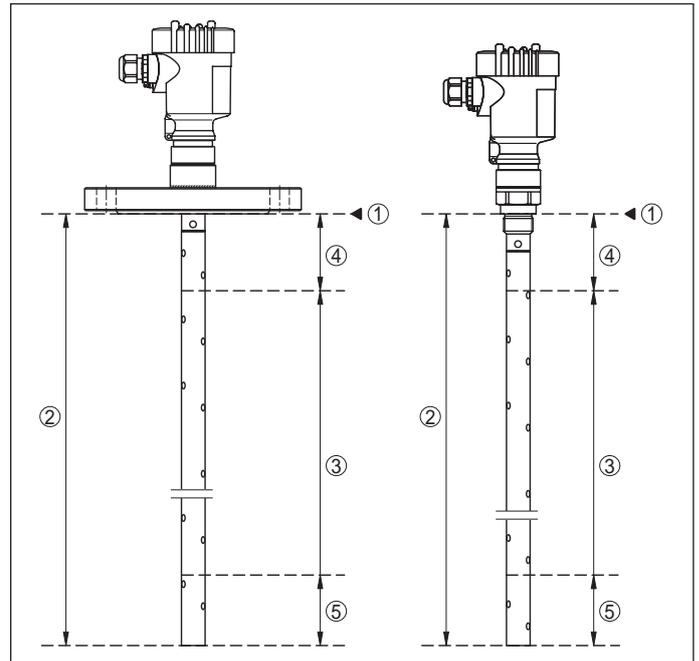
Fig. 2: Measuring ranges of VEGAFLEX - coax version
