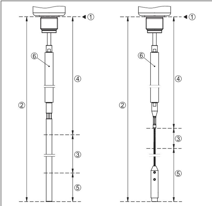
Fig. 19: Measuring ranges - VEGAFLEX with steam compensation
