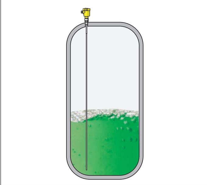
Fig. 28: Level measurement in a storage vessel with VEGAFLEX 81
