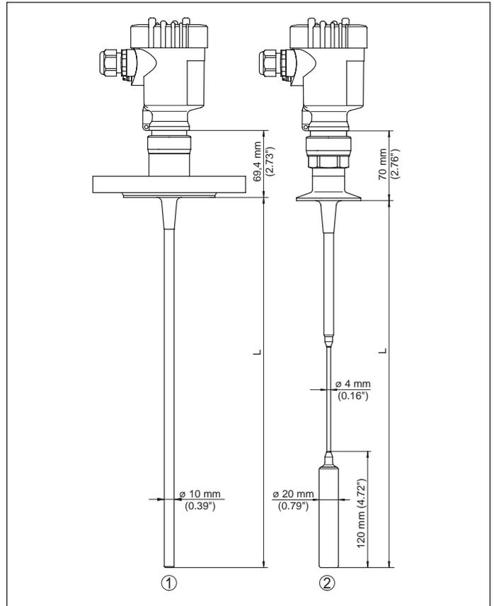
Fig. 56: VEGAFLEX 83, PFA coated version
