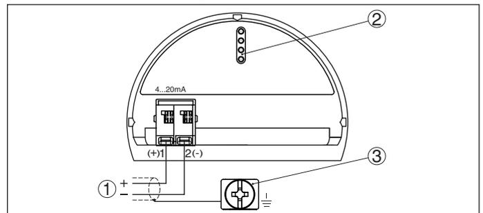
Fig. 32: Terminal compartment, double chamber housing
