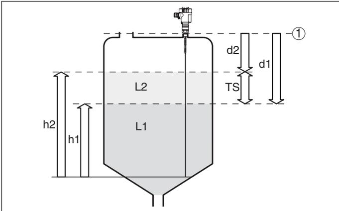
Fig. 15: Interface measurement
