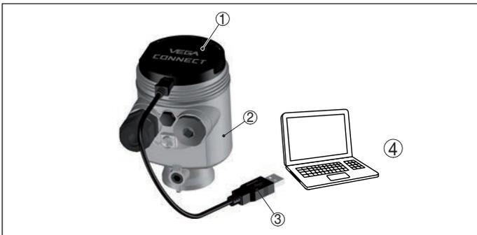
Fig. 44: Connection of the PC via VEGACONNECT and USB
