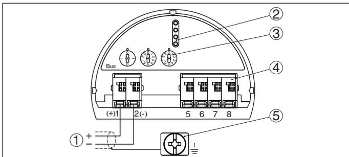
Fig. 35: Electronics and terminal compartment, single chamber housing
