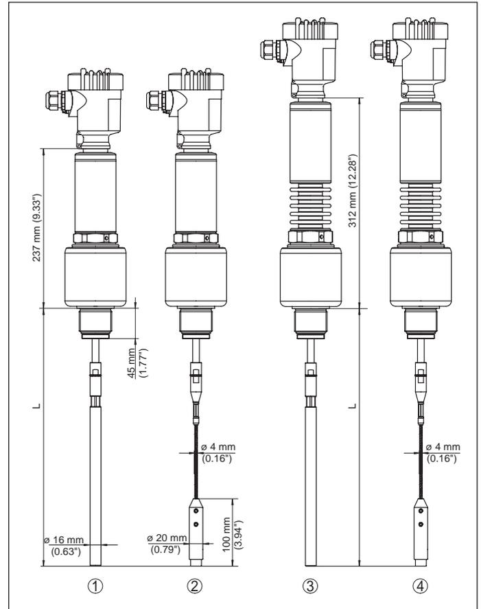
Fig. 58: VEGAFLEX 86, cable and rod version with threaded fitting
