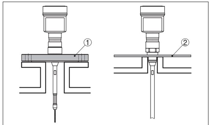
Fig. 18: Installation in non-metallic vessel
