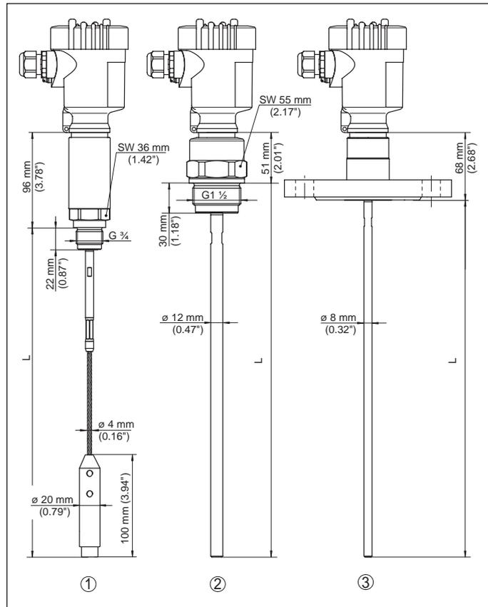
Fig. 54: VEGAFLEX 81, cable and rod version
