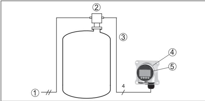
Fig. 47: Connection of VEGADIS 81 to the sensor
