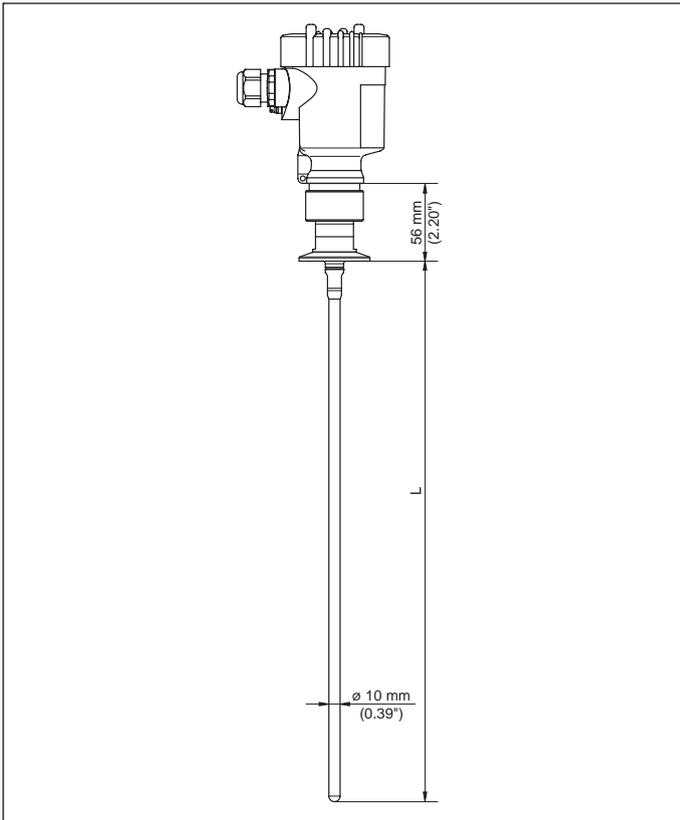
Fig. 57: VEGAFLEX 83, polished version (Basle Standard), rod version  $\varnothing$  10 mm (0.39 in) with Clamp connection
