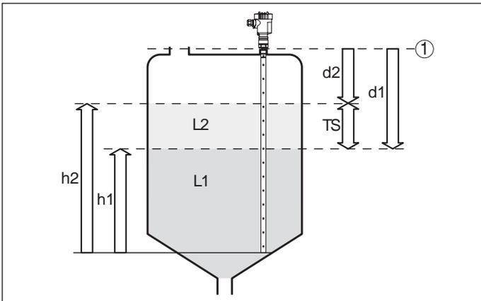
Fig. 3: Interface measurement
