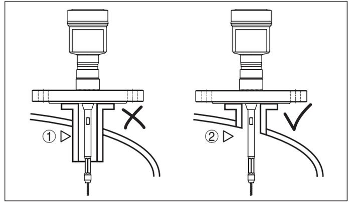
Fig. 17: Socket must be installed flush
