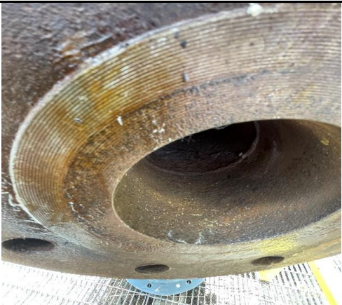
Photo 5: Surface Corrosion on Flange Face
