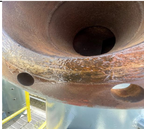
Photo 5: Surface Corrosion on Flange Face
