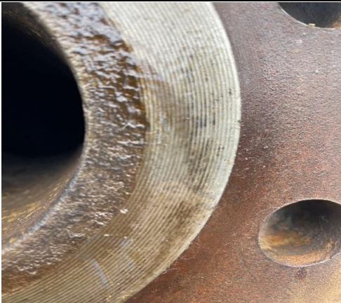
Photo 8: Flange Face Surface Rust
