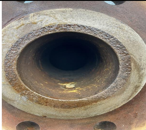
Photo 3: Flange Face Surface Rust
