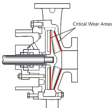
Wear Area Calculation (10 inch dia. impeller)
