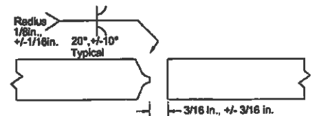
Figure 12 Double J Butt
