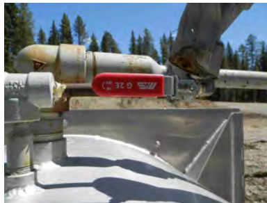
Pilot burner test firing valve
