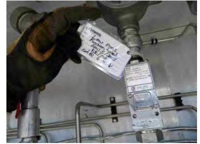
PSLL - Low pressure shutdown
