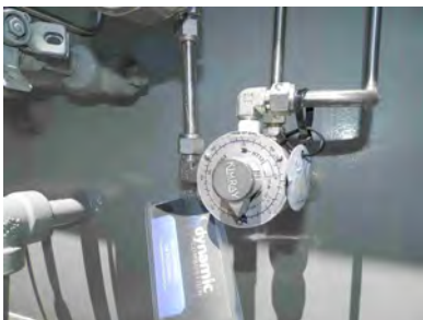
TC - pneumatic process temperature control
