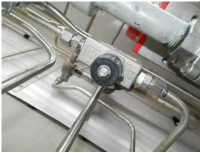
Speed control valve for main SSV
