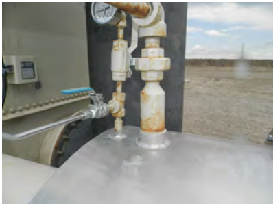
Pilot burner test firing valve
