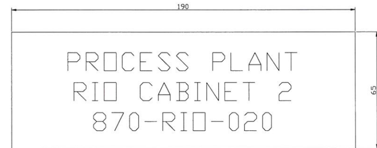
NP1 - CABINET FRONT DOOR NAMEPLATE BLACK TEXT ON WHITE LAMICIDID TEXT SIZE: 10MM
