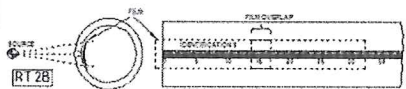
Tech #RT-2B: Long. Weld - Light Wall - Source Outside 1 Exposure/15 inches: QA Subsection 15.12.4
