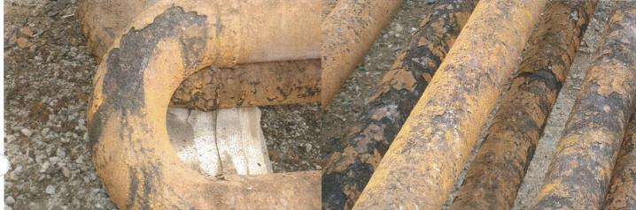
There is light (not measureable) pitting beneath the scale. The tubes have no distortion. Tube sheets have light corrosion and scale. Accessible tube-to-tube sheet welds appear sound.
