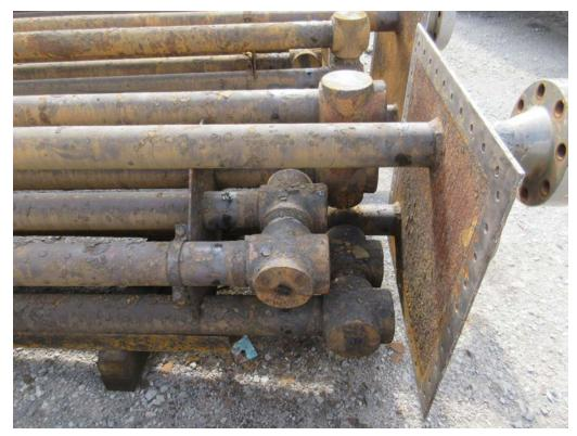
**Condition of Nozzles, Flanges, Repads, and Weepholes:** Nozzles and flanges are in good condition. Coils were pulled out of the Line Heater. There was light chipping on the flanges with minor surface corrosion.
