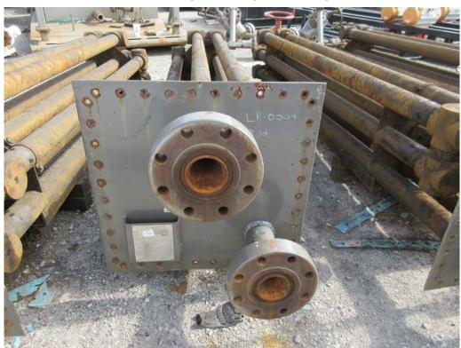
Condition of Welds; Head and Shell Metal Surfaces: The pressure boundary welds have no visual weld defects.
