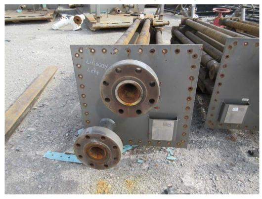
Condition of Welds; Head and Shell Metal Surfaces: The pressure boundary welds have no visual weld defects.
