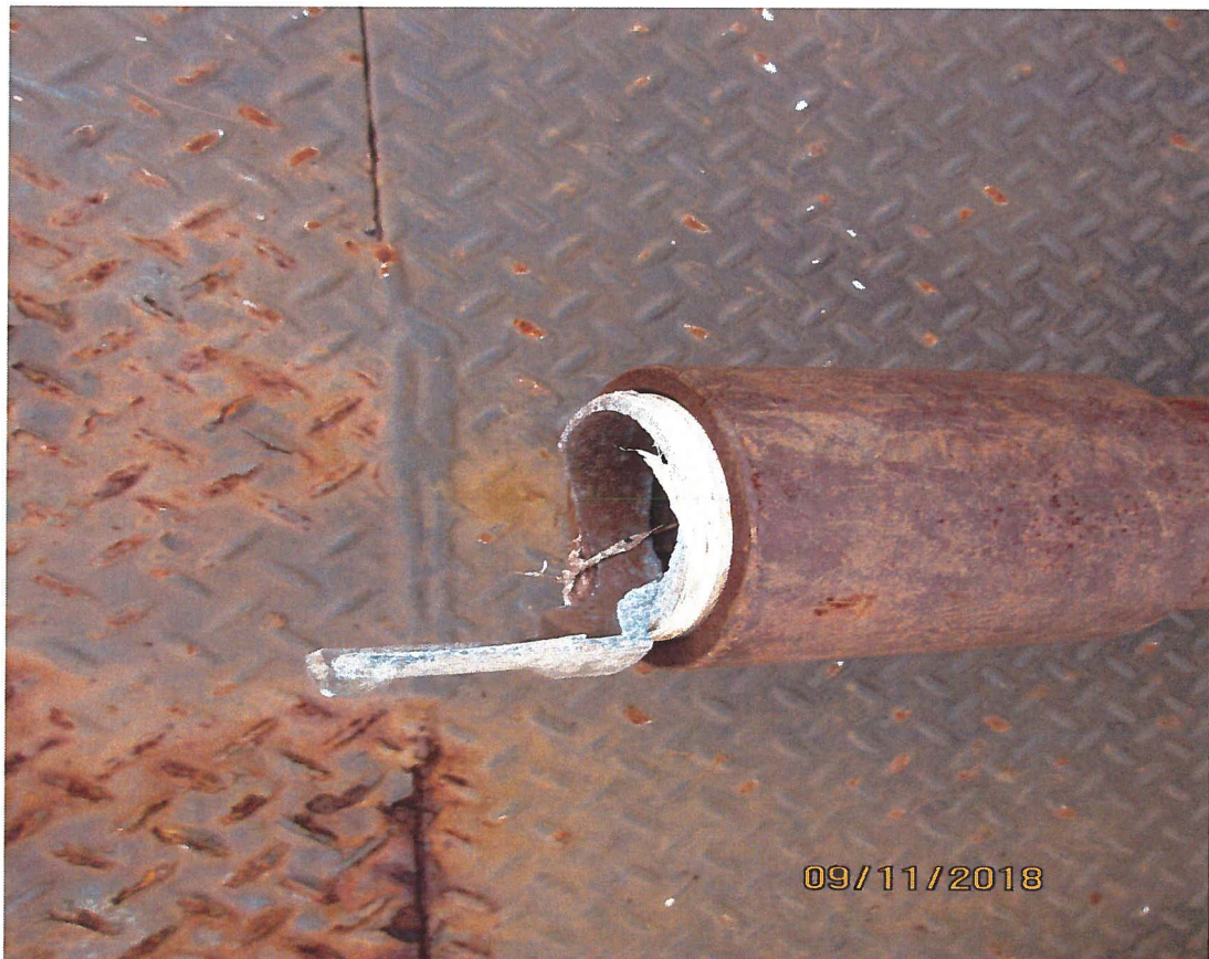
Drain has broken fitting.
