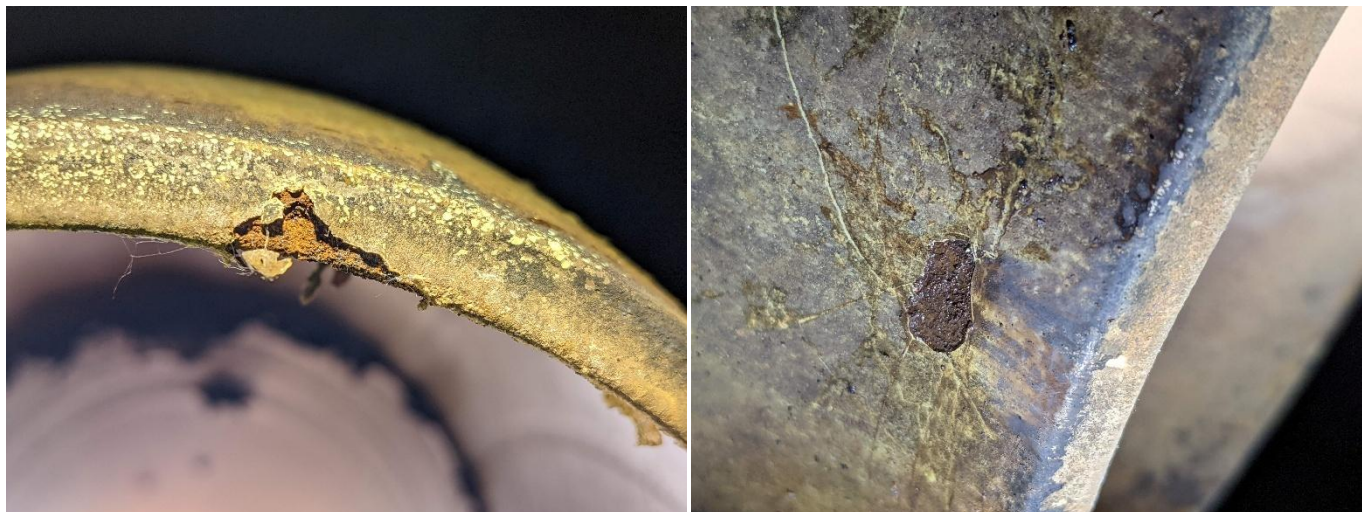
Figures 7 and 8 – Coating Holidays on Inlet Nozzle
