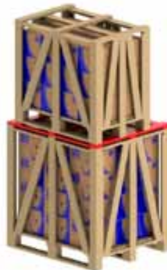
Figure 5.5 – Use of additional battens for stacking
