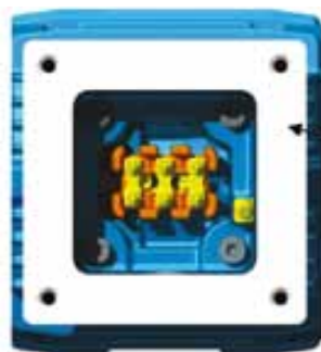
Figure 8.2 - Machined surface of the terminal box of explosion-proof Motors.
