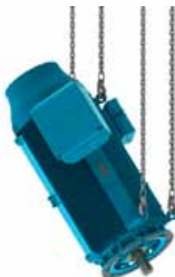
Figure 4.13 – Placing HGF motor in vertical position
