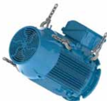
Figure 4.18 – Motor is being rotated to horizontal position
