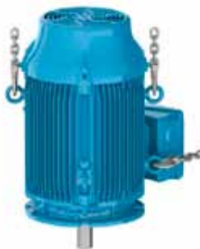
Figure 4.11 – End result: motor placed in vertical position.
