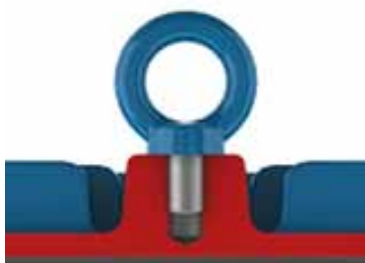
Figure 4.1 – Correct tightening of the eyeboll
