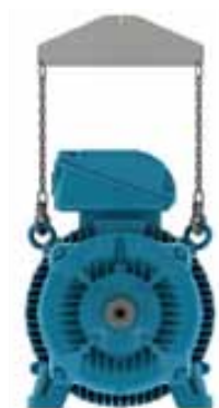
Figure 4.6 – Use of a spreader bar for lifting.
