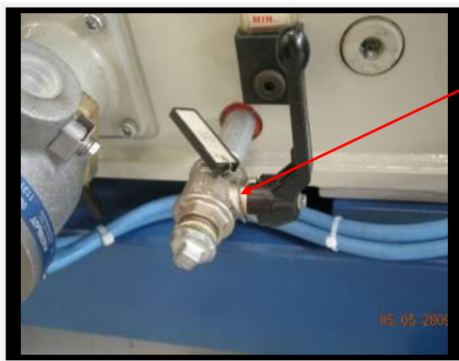
Figure 40 - Oil drain valve example
