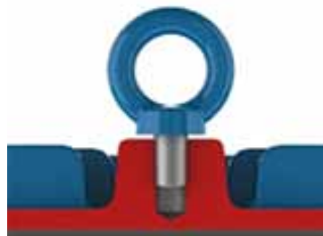
Figure 4.2 – Incorrect tightening of the eyeboll.
