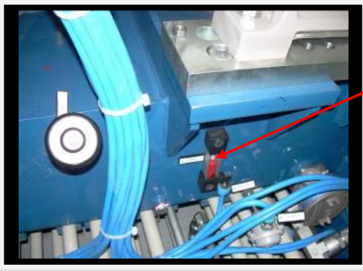
Figure 27 - Level gauge Compressor ST Model
