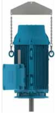
Figure 4.7 – Lifting of vertical mounted motors.
