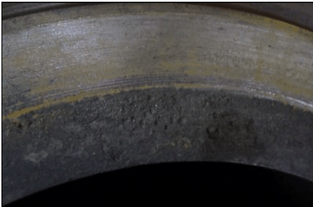
MAN WAY NOZZLE CORROSION
