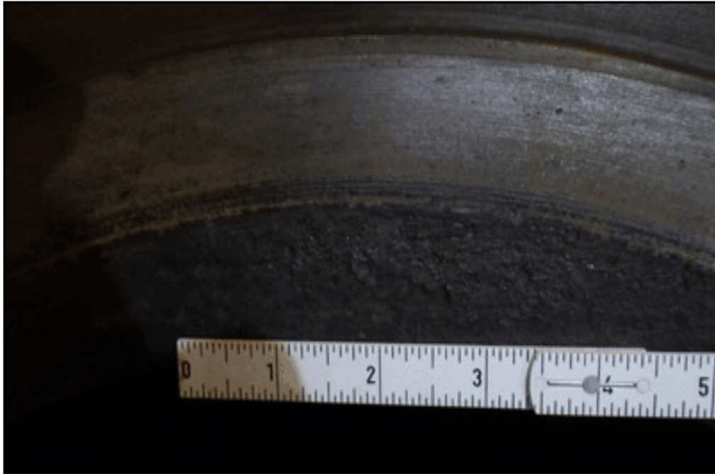
MAN WAY NOZZLE CORROSION
