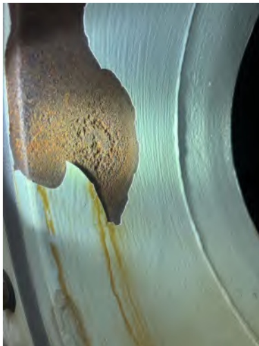
Corrosion on throat measured to a depth of 0.7 mm
