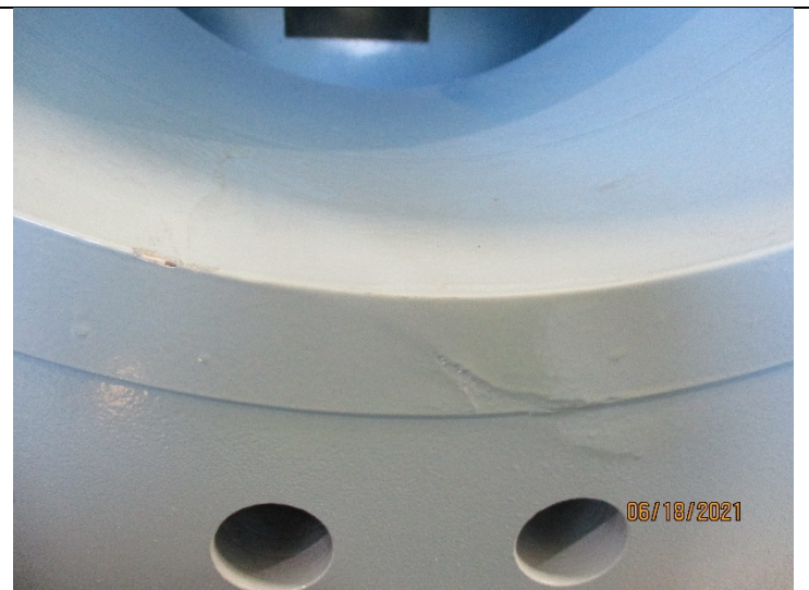
Figure 2. damage to manway coating, seal face. To be repaired by Aspire May 19 2021
