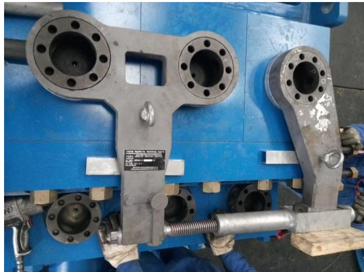
Figure 25: Valve Cover Installing Tool
