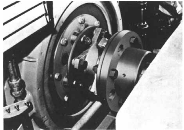
CMR coupling between engine and reciprocating compressor.
