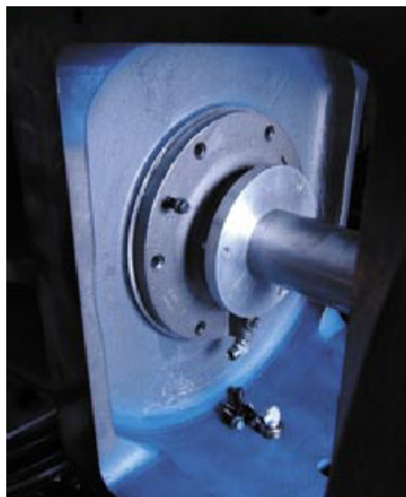
FIGURE 5-3 LOOSENING & REMOVING SEAL HOUSING & TOOL
