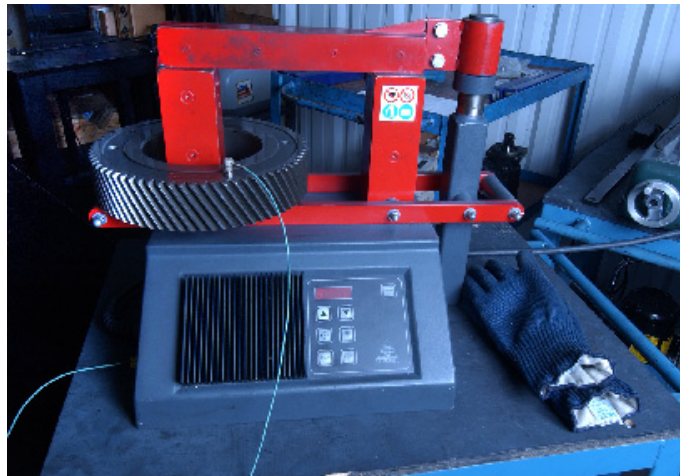
FIGURE 5-23 HEATING NEW GEAR
