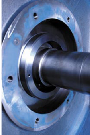
FIGURE 5-4 ROTATING HALF OF SEAL REMOVED
