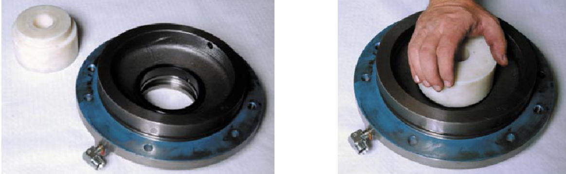
FIGURE 5-6 INSTALLING STATIONARY HALF OF SEAL
