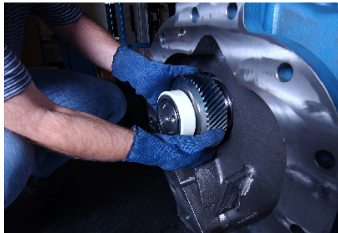
FIGURE 5-24 INSTALLING NEW GEAR
