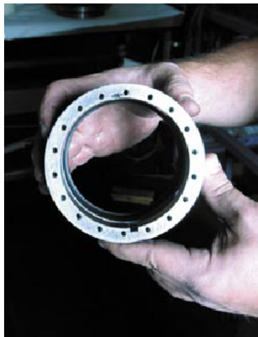
FIGURE 5-5 REAR VIEW ROTATING HALF OF SEAL
