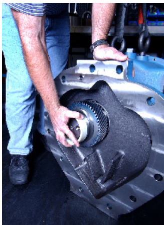
FIGURE 5-18 INSTALLING PLASTIC PROTECTIVE SLEEVE TOOL
