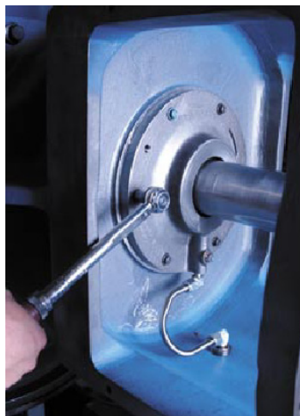
FIGURE 5-7 INSTALLING SEAL HOUSING & TUBING
