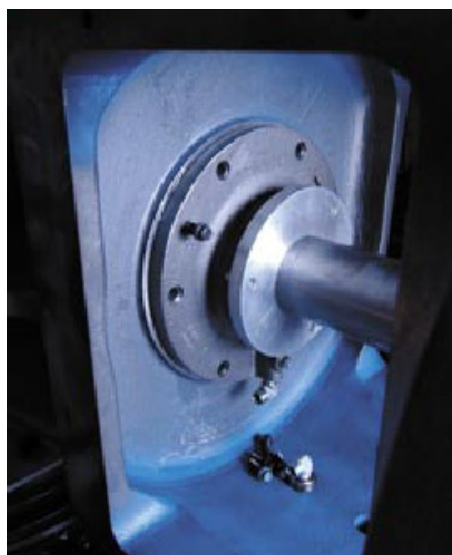
FIGURE 5-3 LOOSENING & REMOVING SEAL HOUSING & TOOL
