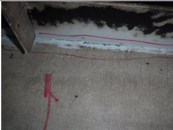
Bottom of fireube throat coating failures
