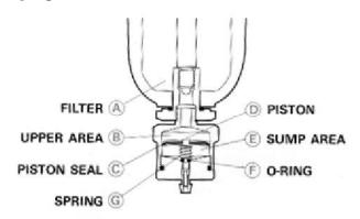
When air flows through filter (A), pressure in upper area (B) equals pressure in sump area (E) and is slightly lower in both areas than filter inlet line pressure (due to friction in flow path). When air flow stops, pressure in (B) increases to equal inlet pressure, and forces liquid past piston seal (C) into (E) until (B) and (E) both match inlet pressure.
